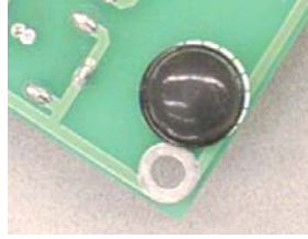
Figure 1-21 Rubber Feet (left) Affixed to Underside of the Board of Education (right)
